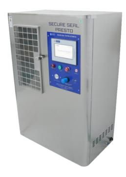
Secure Seal Tester – Next Generation Model is a consistent tool useful to measure the thread and seal integrity on bottles either Pet or Glass. The bottle secure seal tester has been designed to address the special needs of sealing beverage containers that use various seals, such as aluminum roll-on, twist crowns. By detecting gas leakage rather than liquid, the Secure Seal Tester gives more sensitive, accurate readings.
